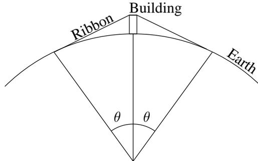
Figure 3. Once on the ground, the ribbon pushes down on objects that protrude along its path.
