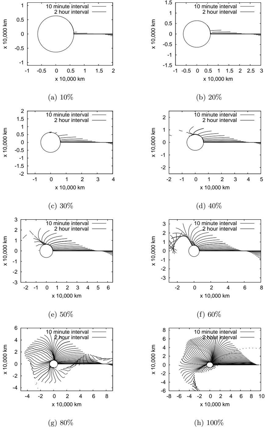
Figure 2. Space elevators falling back to Earth after being severed at different heights, seen from above the North pole.
