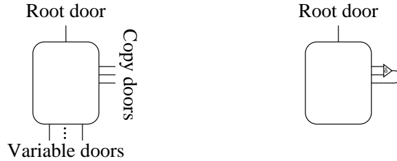
Figure 3.3: On the left is a net that is being built. It still has free variables, and it has a port through which it makes copies. On the right is a net that has been finalized by putting a copy operator (a \delta agent) on its copy port. Note that the finalized term has no variables. Indeed, the terms that would be plugged into the free variable ports must be \delta -free and there is no room left to connect the variable's copy port. It would be possible to leave room for each free variable to have a copy port. For simplicity, and without loss of expressive power, I will only consider finalized terms without any free variables.
