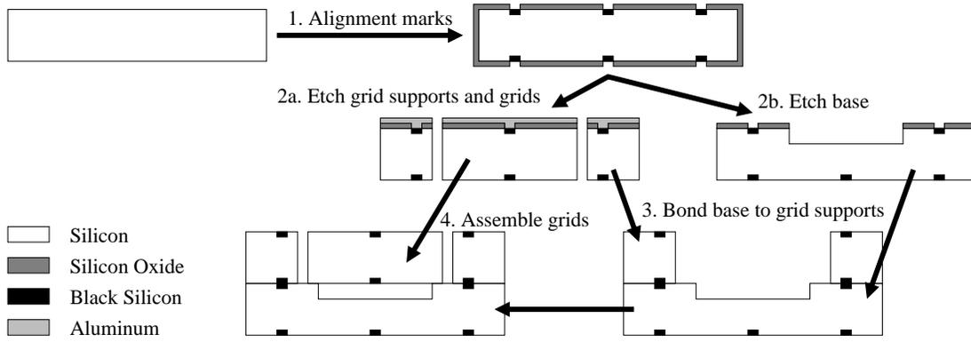
Figure 8. Fabricating the test device.
