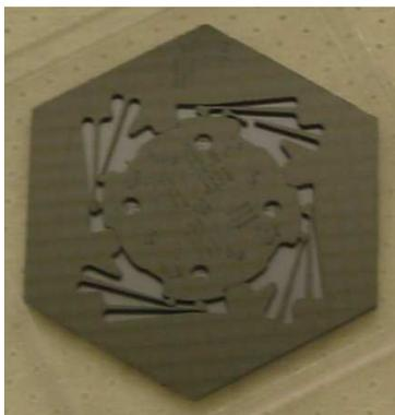
Figure 9. An assembled grid with a broken finger.
