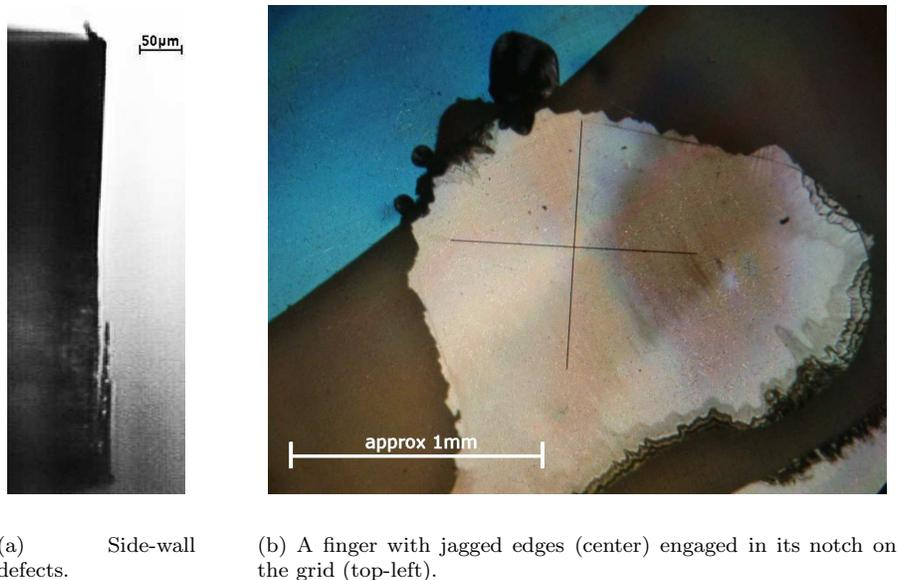
**Figure 11. Some processing defects in the finished devices.**
