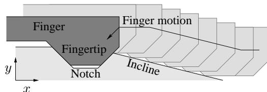
Figure 4. The motion a finger follows during assembly.
